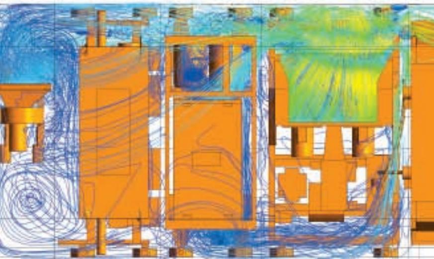
Pathlines (colored by velocity) through the traction component hardware
