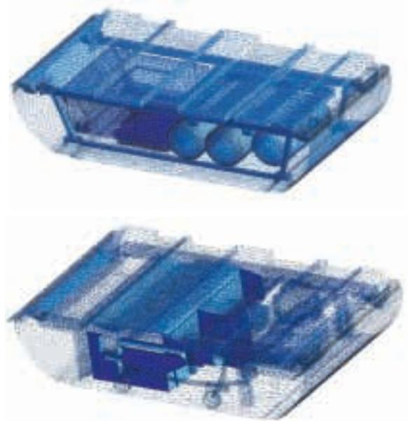
Complex meshes of different traction components generated by ANSYS ICEM CFD meshing software
